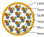
LSOH (SHF1) Outer Sheath Tinned Copper Drain Wire XLPE Insulation Al/polyester Tape Screen Mica Glass Tape Stranded Copper Conductor
